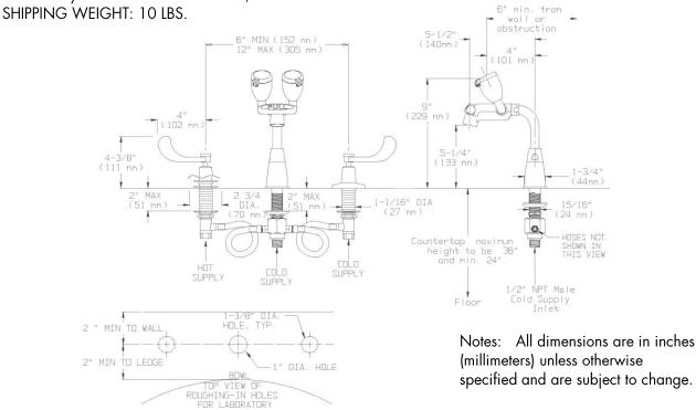
**IMPORTANT:** The supply line for plumbed units shall provide an uninterruptible supply of flushing fluid at a minimum of 30 psi . of flow pressure. If shut off valve are installed in the supply line of the eyewash for maintenance purposes, provisions shall be made to prevent unauthorized shut off.
